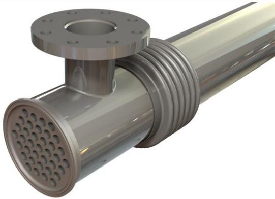
The HRS MI Series is complete stainless steel shell and tube design for food industry use. The product flows through the interior tubes and the media fluid flows through the surrounding shell. The MI Series is an ideal heat exchanger for pasteurisation applications. Using HRS corrugation technology, both heat transfer and efficiency are increased over standard smooth tube heat exchangers. In addition potential fouling is minimised.
